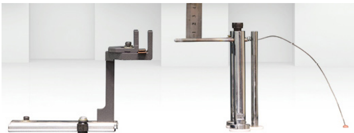
Glow Wire Testing Apparatus Used to Evaluate Different Resins
