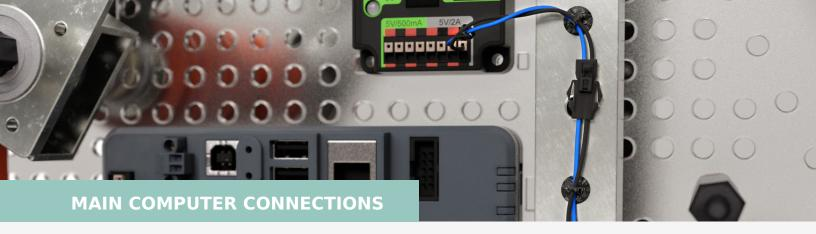
Signal connections could have purposes ranging from running the serial peripheral interface (SPI) to connecting to your RoboRio™ (main controller). While many connections in these systems require a stripped wire that is inserted into a terminal block some may have pin headers that can use the Molex SL connection systems. For wire-to-wire applications, we advise adopting a more enhanced connection system.
