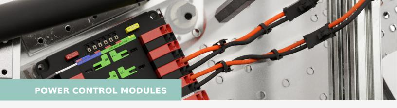
Power control modules may be used from multiple approved companies in the FIRST Robotics guidelines. We typically see these modules using larger wires that range from 8 to 12 AWG. These cables generally have leaded wires but may be updated to allow for wire-to-wire applications.
