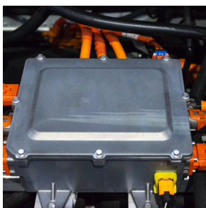
Battery Management System
